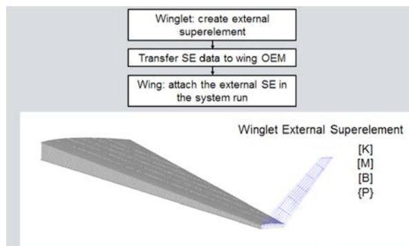
Figure 1: Winglet external superelement.
