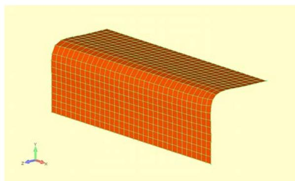
Figure 9: Refined mesh fitted through rebuilt surface.
